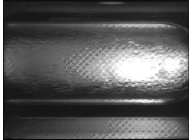
Figure 4. Annular flow pattern of pure ammonia flowing at x = 81\% and G = 122 \text{ kg} \cdot \text{m}^{-2} \cdot \text{s}^{-1} .
